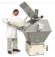
Minimize housekeeping and air-quality problems with optional dust collection hood. Keeps material in process; makes work environment safer.
